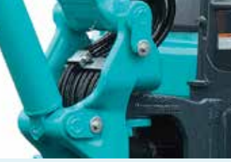
Hydraulic piping The hydraulic piping is housed inside the swing bracket.
