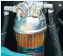
Pre fuel filter with built-in water separator
