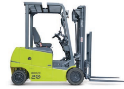
Bravo 4 wheel electric forklift 1.5 / 2.0 tonne
