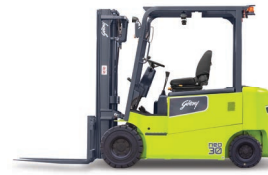
Neo series electric forklift 1.5 / 2.0 / 2.5 / 3.0 tonne
