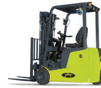
Bravo 3 wheel electric forklift 1.6 / 2.0 tonne
