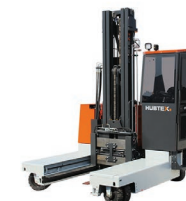
Side loader MQ series up to 35 tonne
