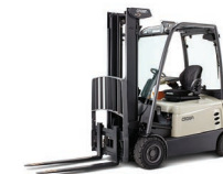
SC 6000 series electric forklift 1.4 / 1.8 / 2.0 tonne
