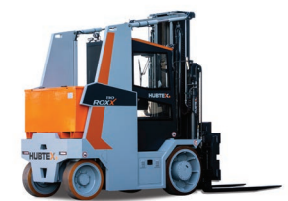
Compact heavy electric forklift up to 30 tonne
