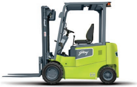
Lithium-ion forklift 2.0 / 3.0 tonne
